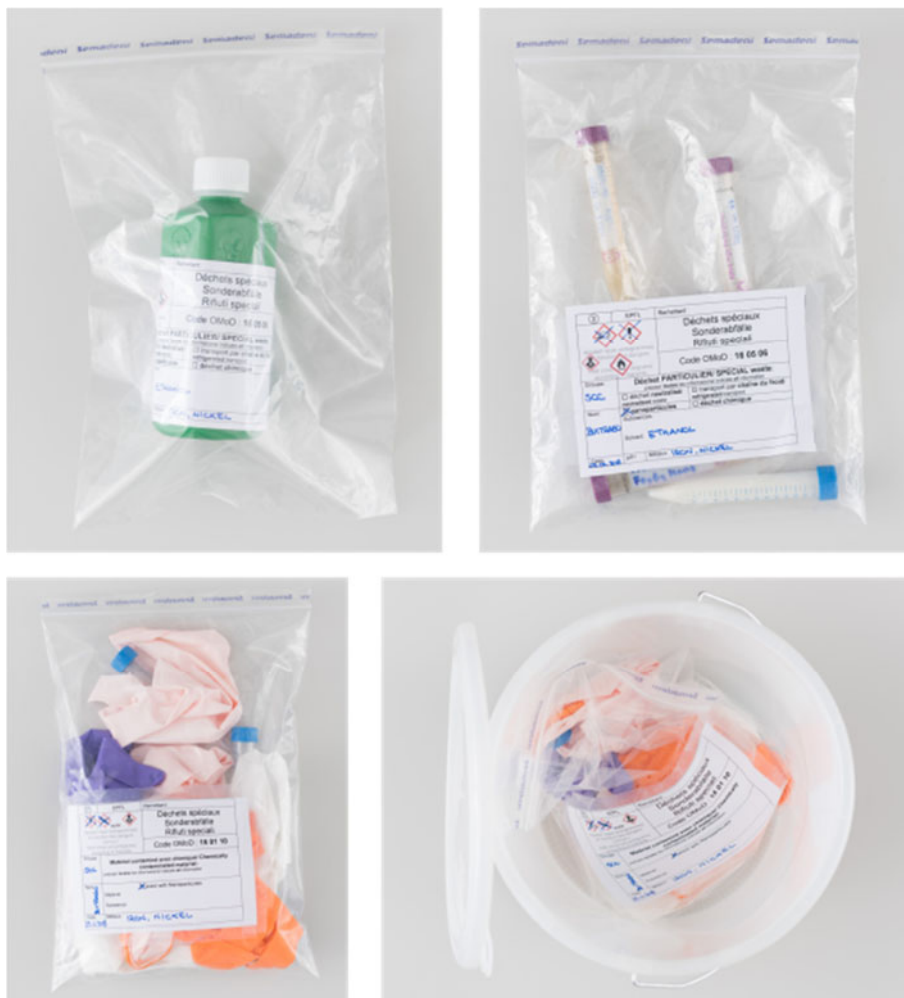
Figure 6: Double packaging of nanomaterial waste.
