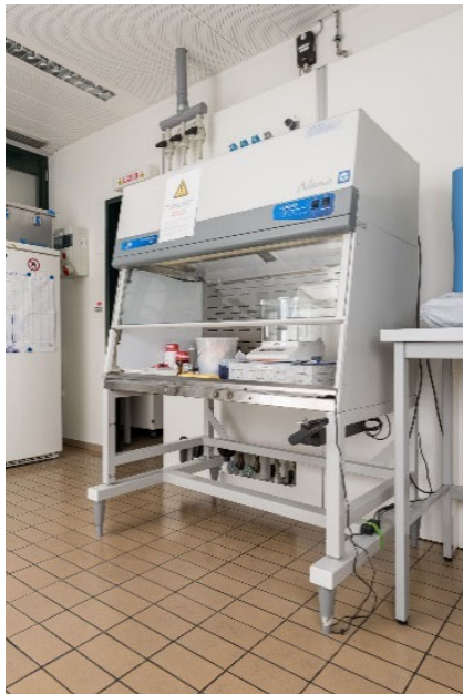
Figure 2: Nano enclosure designed for work with fine powders.
