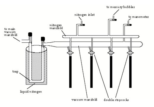
The designs of Schlenk lines vary in individual labs. For example, at EPFL, we are not allowed to use mercury bubbler, so we use a silicon oil bubbler. We use a digital vacuum manometer to monitor the vacuum, whereas in most places in the US Hg manometers are common.
