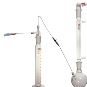
Fig. 13 Double-ended needle transfer with syringe valve
