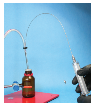
Fig. 8 Filling syringe using nitrogen pressure
