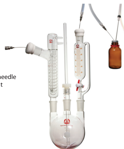
Fig. 13 Double-ended needle transfer with syringe valve
