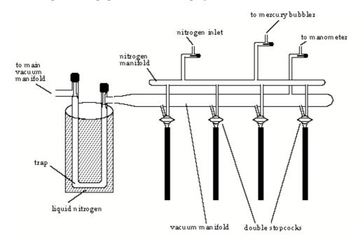
The designs of Schlenk lines vary in individual labs. For example, at EPFL, we are not allowed to use mercury bubbler, so we use a silicon oil bubbler. We use a digital vacuum manometer to monitor the vacuum, whereas in most places in the US Hg manometers are common.
