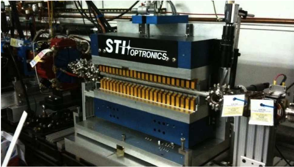
Figure 25: The second undulator after installation in beamline.
