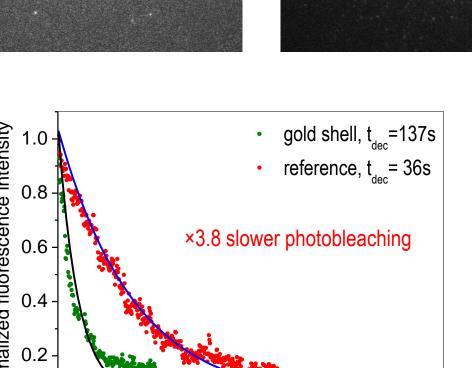
Comparison of fluorescence photoresistance against photobleaching for calcein-loaded vesicles and hollow gold containers (plasmon resonance set at 590 nm).
