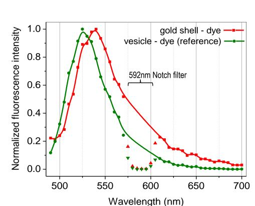
Plasmon field enhancement affects the fluorescence lifetime of a dye [6, 9], resulting here with about 20 nm broader Stock's shift of the
