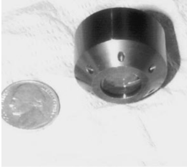
Fig. 3. Picture of the imaging lens designed for HROM.
