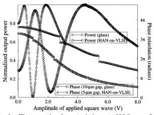
Fig. 2. Electro-optic characteristics at 632.8 nm of a transmissive HAN cell with a 10- $\mu$ m gap and a reflective HAN-on-VLSI sample with a 5- $\mu$ m gap. Both cells were filled with Merck E7. Note that the entire amplitude-modulation range of the HAN-on-VLSI device is spanned by the 1.1-V amplitude interval between 1.1 and 2.2 V.
