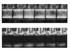
Fig. 3. Rows of six pixels at maximum (top) and minimum (bottom) reflection settings. Voltage-dependent reflectance is also observed in the areas surrounding the pixels, as a result of the presence of conductors at various potentials and depths within the silicon dioxide.
