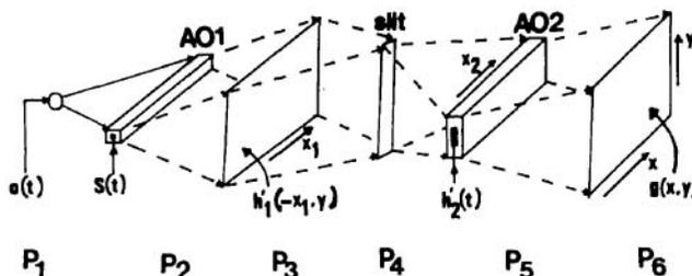
Fig. 1. Acousto-optic image-processing system. AO1 and AO2 are acousto-optic lines,  $P_2$  is imaged onto  $P_3$  in the horizontal direction,  $P_3$  is imaged onto  $P_5$ ,  $P_4$  is a pupil plane,  $P_5$  is imaged onto  $P_6$ , and  $P_6$  is the detector plane.
