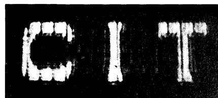
Fig. 5. Image used for PR correlator experiments. The photograph was taken from the disk by using the diffractive readout scheme described in Ref. 1.
