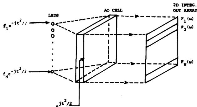
Fig. 2. Schematic diagram of a multichannel electrooptical Fourier transform system for advanced Fourier spectroscopy signal processing.
