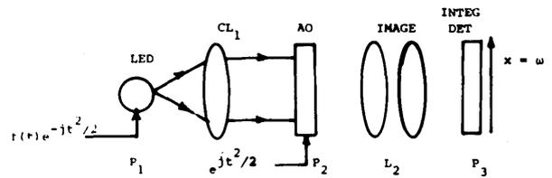
Fig. 1. Schematic diagram of a time-integrating chirp-Z acousto-optic Fourier transform system.
