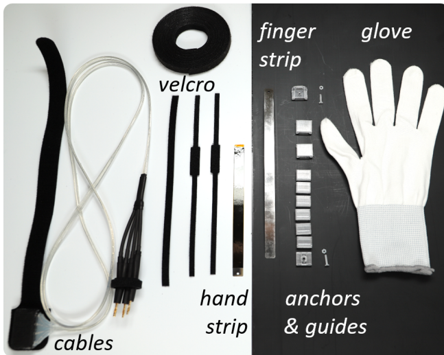
Figure 4. Assembly of the ES brake, 3D printed guides and attachments fastened to thin nylon glove using velcro.
