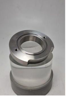
High pressure oedometric ring developed by Héloïse Fuselier for thermo-mechanical testing
