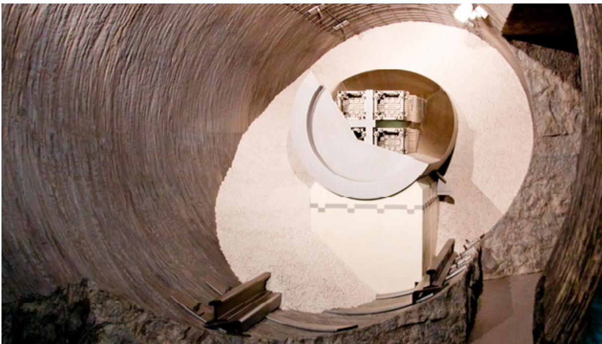
A simulation in Grimsel granite shows the uranium rods, the steel container and the buffer layer of bentonite
