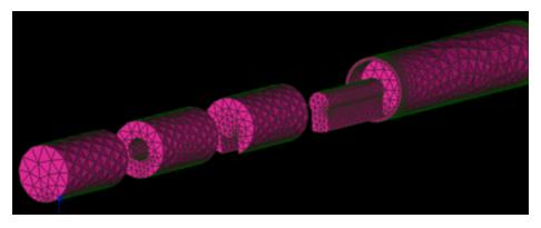
Finite Element model: containers, bentonite blocks and hydraulic seals (from René Carpaij's project)
