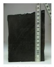
Example of gas shale core sample retrieved at thousands of meters depth
