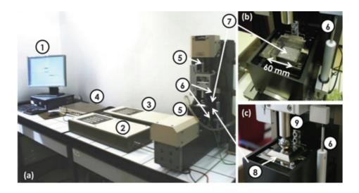
Original version of the GDS direct shear device: (a) global view, (b) detail of the open shear box, and (c) detail of the closed shear box. 1, GDSLAB software control; 2, normal actuator; 3, horizontal actuator; 4, LVDTs acquisition pad; 5, load cells; 6, LVDTs; 7, specimen placement; 8, top cap; 9, axial piston (Di Donna, Ferrari and Laloui, 2015).
