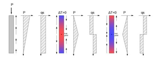
Behaviour of a pile subjected to mechanical and thermal loads. Source: Rapport Etienne
