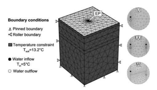
Example of three dimensional finite element model used to investigate the energy, geotechnical and structural performance of energy piles for different design solutions (Batini et al., 2015).
