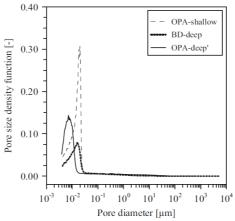
Pore size density function of some tested shales by LMS
