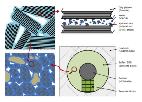
Looking at nuclear waste storage at different scales. The buffer of the deposit is made of a porous clay matrix with some impurities. The clay matrix itself can be seen, at a smaller scale, as an arrangement of stacks of mainly smectite platelets
