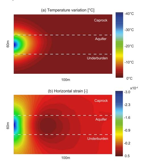
Spatial distribution of (a) the temperature variation and (b) horizontal strain after four years of injection
