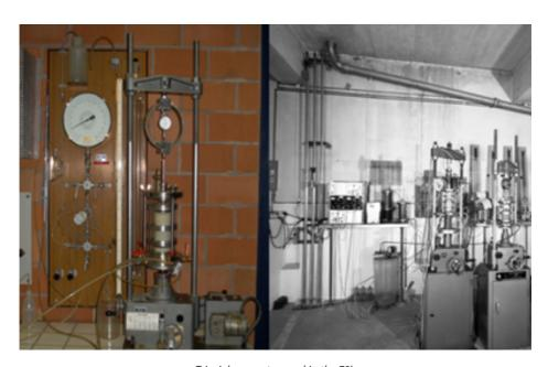
Triaxial apparatus used in the 70's
