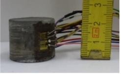
Setup for anisotropic volumetric response of shales upon saturation/desaturation cycles
