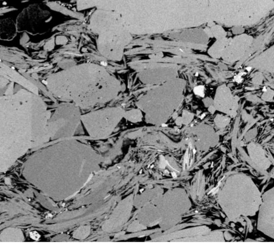
SEM image of a gas shale polished specimen. The figure highlights the complex and heterogeneous structure composed of carbonate grains, clay particles and organic matter
