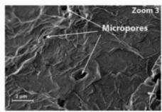
Scanning electron microscopy images of sand/bentonite mixture
