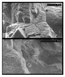
Growth of calcium carbonate crystals (Cubis shaped, plane expansion) on the surface of grains
