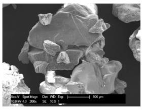
Calcium carbonate particles bridging soil grains as a result of soil bio-cementation (surface analysis via Electron Microscopy)
