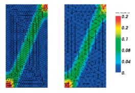
Damage-plastic model : damage distribution for a finer mesh (left) and for a coarser mesh (right)
