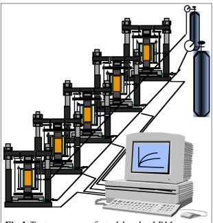
Fig.1 Test set-up perfected by the LRM to carry out 5 simultaneous identical triaxial creep tests.
