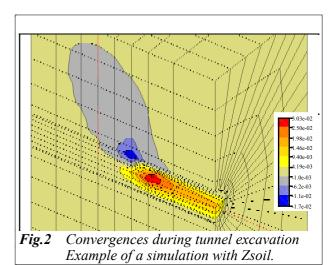
Several laws are included in the finite element code ZSOIL<sup>3</sup> and have been verified using in situ measurements from real constructions (Figure 2).
