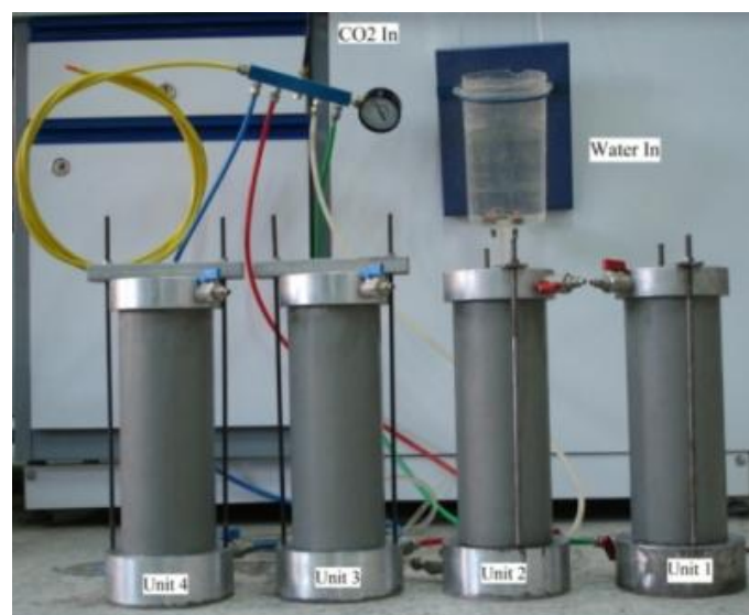
Figure 1- Cementation units for four sample preparation.
