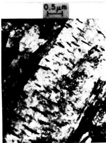
Figure 2-24 Precipitation of Fe_3C in Fe-0.39% C martensite tempered 1 h at 300°C. (Electron micrograph.) [After G. R. Speich and W. C. Leslie, Met. Trans. 3(1972):1043.]
