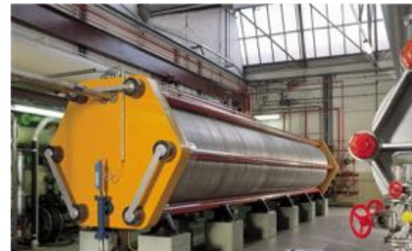
Alkaline Electrolyzer 4MW, 1980 Giovanola, Lurgi, IHT
