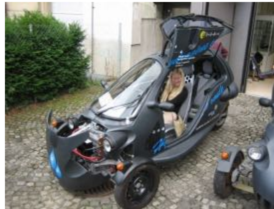
FC vehicle MH storage 0.5 kg H 2 , 1.2 mass%
