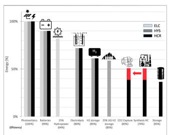
**FIGURE 6** | Efficiency loss along the conversion chain (light gray for substitution of fossil fuels through electrification (ELC), dark gray for substitution of fossil fuels by hydrogen (HYS), and black for substitution of fossil fuels by synthetic hydrocarbons (HCR)] relative to the electricity produced by photovoltaic (PV) (100%).
