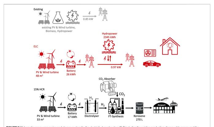
FIGURE 9 | Schematic energy conversion and storage system for the electricity-based system ELC including the existing production of renewable energy and the production of synthetic hydrocarbons as jet fuel (per capita).
