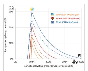
**FIGURE 7** | Necessary energy storage capacity (S) as a function of the annual PV production ( $PV_y$ ) in relation to the annual energy demand (**Figure 3A** line, **Figure 3B** dotted line). The curves maximum represents the seasonal storage and the minimum limit is a day/night storage of 0.25% of the annual energy demand.
