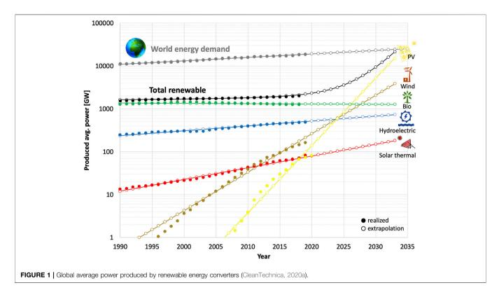
the global energy demand of  $24\,\mathrm{TW}_\mathrm{p}$  will be reached by the average power of installed renewable energy in 2032. As can be seen in **Figure 1**, the growth is slowing down in recent years as the fitted line is above the actual installed power for PV, wind, solar thermal, and the sum of all renewables (total); however, it is still growing exponentially.
