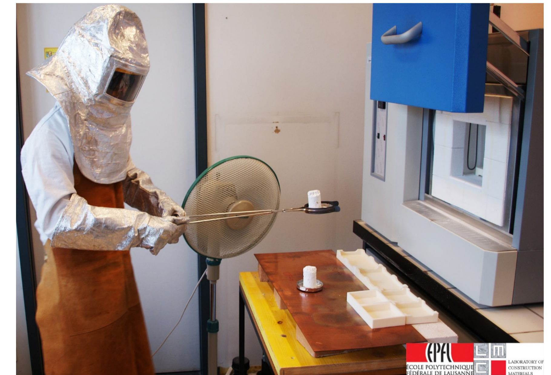
Sample during quenching, a mock sampling at room temperature.
