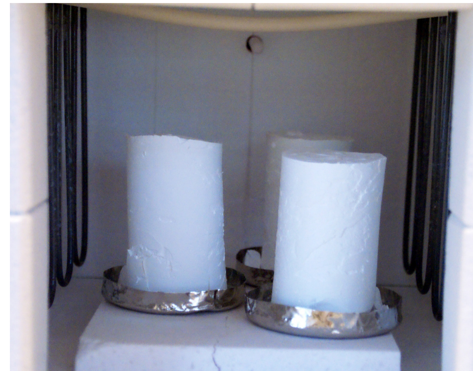
Sintering using dried green cylinder in the furnace
