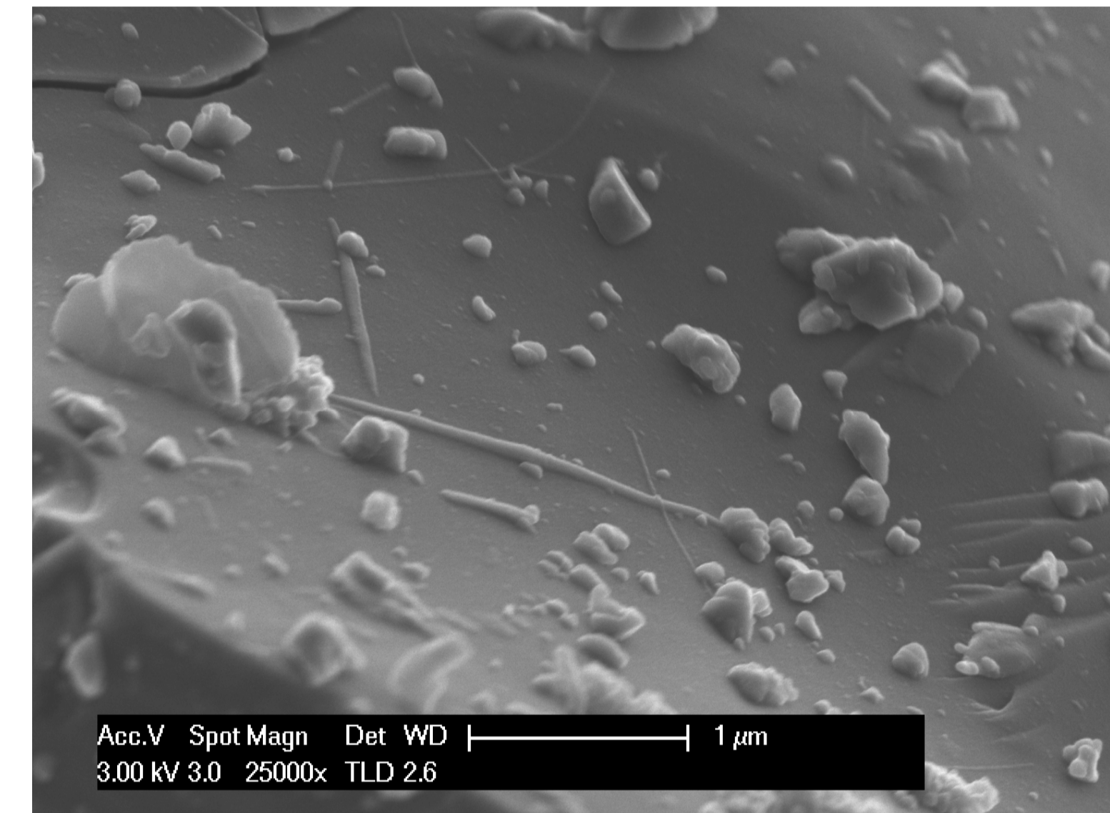
HR-SEM image of alite surface after 1 hour of hydration : nucleation of C-S-H crystals can clearly be distinguished.
