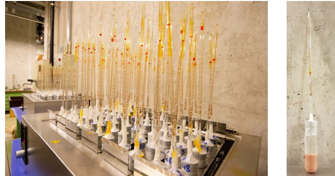
Fig. 1 (a) a chemical shrinkage bath filled with 72 tubes, (b) a single tube + rubber cap + pipette + paraffin film of an LC3 cement.
