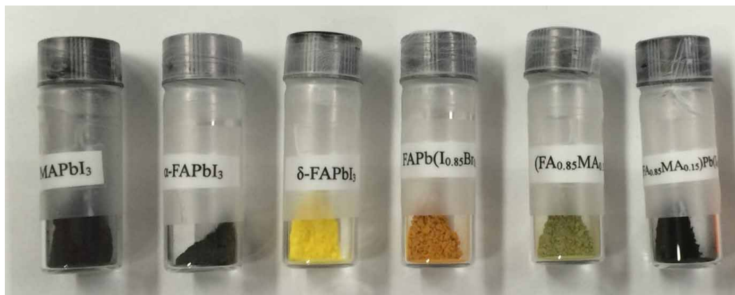
Extended Data Figure 4 | Photographs of inorganic-organic hybrid halide powders. Photographs show the colour of the as-prepared MAPbI 3 , annealed FAPbI 3 at 170 °C, FAPbI 3 , (FAPbI 3 ) 1-x (MAPbI 3 ) x ,
