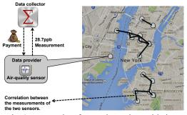
**Figure 1:** An example of crowdsourcing with incentives: Crowd-sensors (*air-quality eggs*<sup>1</sup>) report air-quality measurements and a data collector rewards them with monetary payments. An edge (black line) indicates that there is a sufficient correlation between the measurements of two sensors to verify accuracy.
