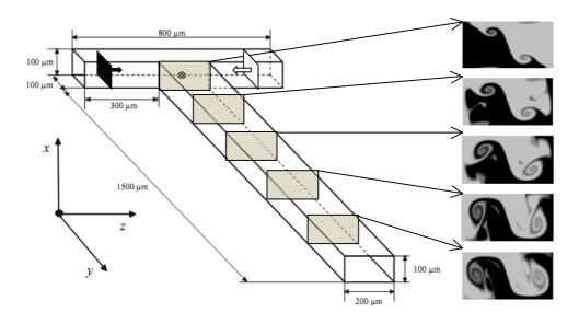
Fig. 1 Mixing in a T junction (Carsten Stemlich, PhD Thesis, Erlangen)
