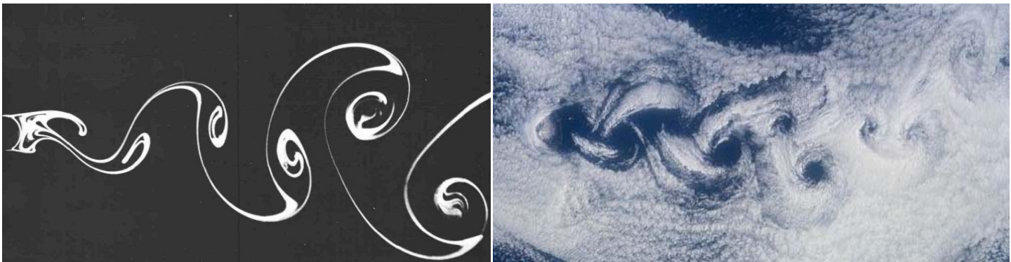
Von Kármán vortex street. Left: downstream a circular cylinder, Re=140 [Taneda]; right: downstream the volcanic island of Rishiri in Japan [NASA].
