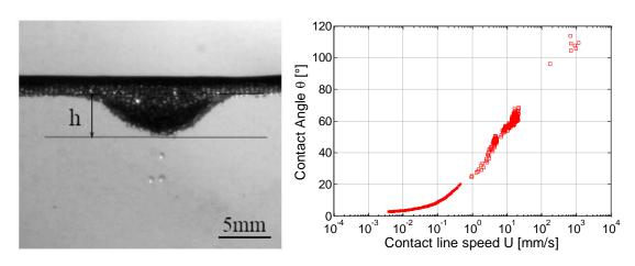
**Left:** Spontaneous impregnation of a floating island of non-soluble grains [1]. **Right:** Dynamic wetting angle of a water droplet on a maltodextrin thin coating [2].
