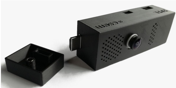
Glare Meter integrating an HDR vision sensor and an Intel Compute Stick for on-the-fly glare and workplane illuminance assessment with WiFi data transmission..
