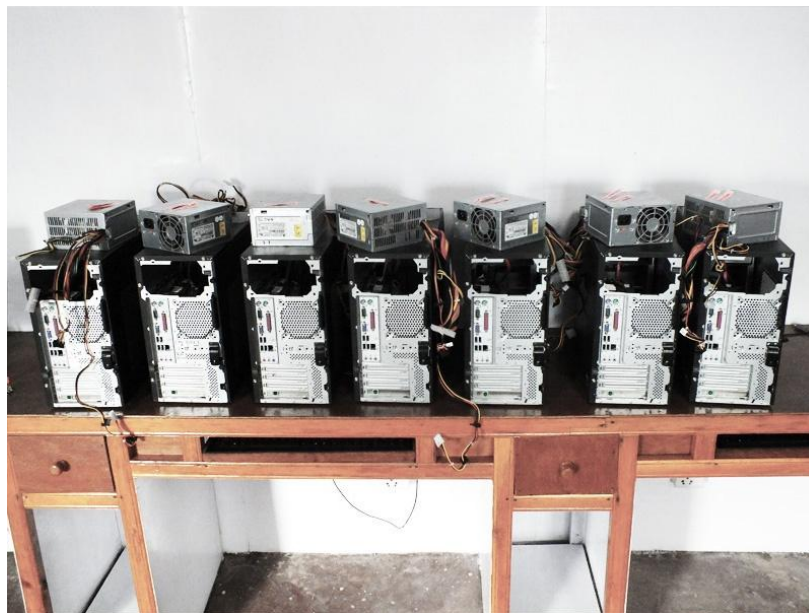
Figure 54: Seven power supplies that need to be replaced (4).
