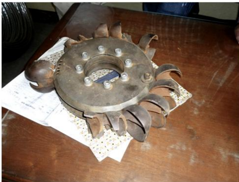
Figure 4: Pelton runner (spheroidal cast iron) destroyed after approximately after 4,000 working hours (9).
