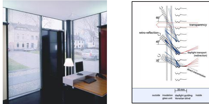
Fig.2.8: Retrolux blinds with a very interesting geometry that permit the daylighting control.
