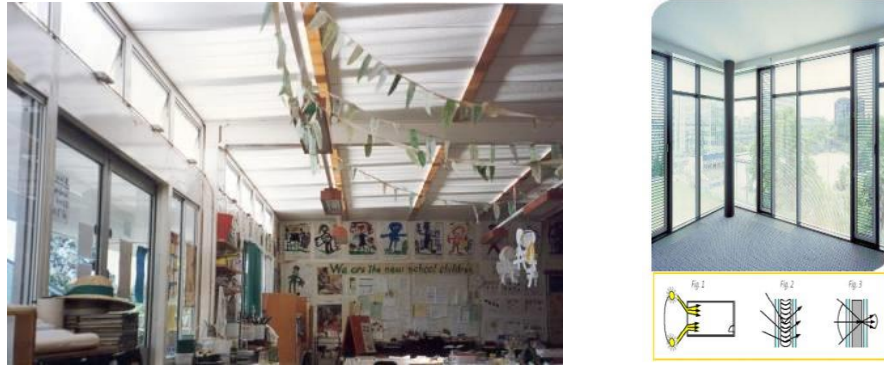
Fig.2.10: (a) Solartran laser cut panels in a classroom installed in the top part of a window (b) Lumitop glass Saint Gobain.
