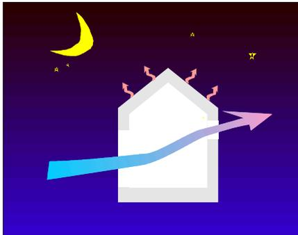
During the night the building is naturally ventilated at a maximum rate in order to remove the heat and to cool the internal side of the walls. These cool wall surfaces provide comfort during daytime.
