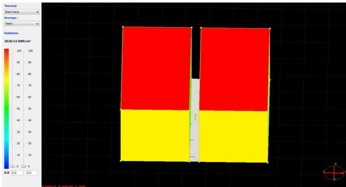
Figure 138 Orientation North-South, distance between buildings 2 [m]. Solar irradiation, yearly results. Max value 2020 [kWh/m²]. East view.
