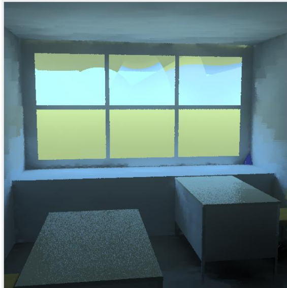
Figure 19: View of the visualization area of the GERONIMO interface (middle-section) showing a picture created using the rpict command.
