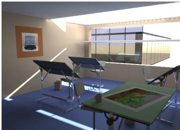
Figure 1 : Radiance lighting simulation of a Light Shelf day lit office space (Greg Ward 1994).
