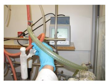
Step 3 Close the flask, warm up the solvent until everything is liquid again (obviously keep the flask closed, you are still under vacuo!). You can use a water bath to accelerate this process. To promote a better gas exchange, you can shake it a bit and you should not fill the flask more than 50% (the picture is therefore
