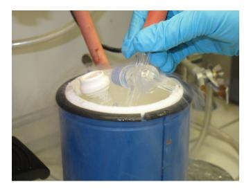
Step 2 Put the flask under vacuo (<0.5 mbar).
