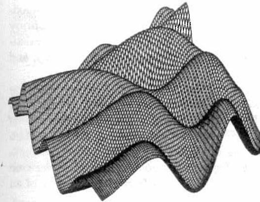
FIGURE 2.6 It is often useful (but sometimes dangerous) to think of the energy as something like this landscape. The z -axis is the energy and the 2^N corners of the hypercube (the possible states of the system) are formally represented by the x - y plane.
