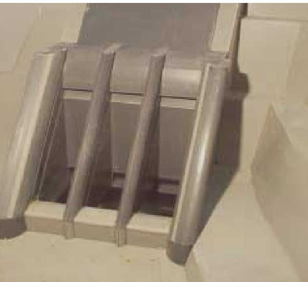
Fig.2. Front view of the intake model 1:20
