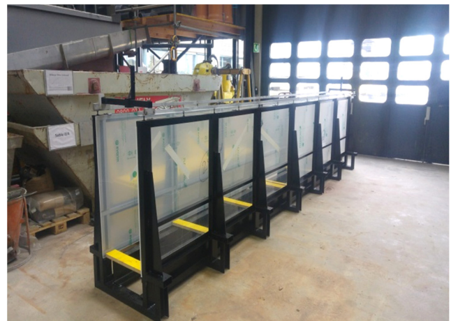
Figure 1: Experimental facility: inlet conditions-jetbox(left), stepped chute(left) and stilling basin(right).
