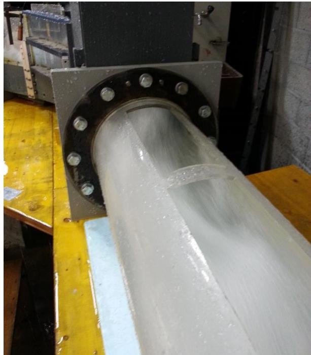
Figure 3 : (left) Impact of shock wave B on the manhole sidewall and (right) downstream view of the shocked flow outing from the manhole, as observed during some test-runs.
