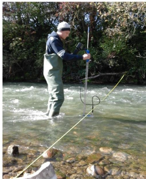
Figure 2: In-stream measurements using a floating ADV (left) and a handheld ADV (right)
