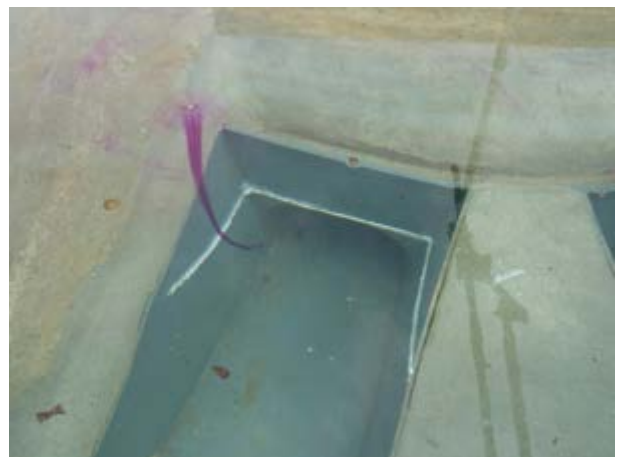
Figure 1 : In/outlet structure on physical model (left : In/outlet structure with a vortex mitigation structure, right : Type III vortex observation)
