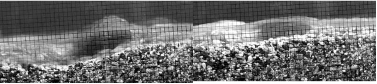
Figure 4 : Rapid variation in boulder protrusion. On the left the boulder at time 0 and on the right the same boulder 5 minutes later (with \lambda/D=5 [-], D=0.125 [m], q=0.0207 [ m^2/s ], q_s=1.40 \cdot 10^{-4} [ m^2/s ])
