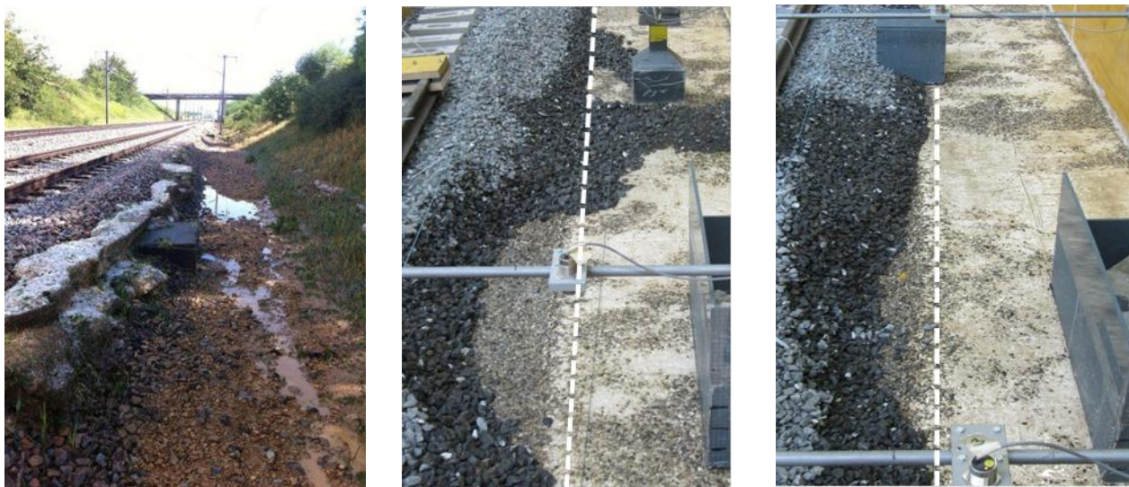
Figure 1 : Left: picture taken after the thunderstorm occurred in Sarry in 2000. Center: test with 2 obstacles, with the catenary pole downstream of a bridge pier. Right: test with 2 obstacles, with the drainage manhole downstream of a bridge pier. Distance between obstacles for the presented tests is 4.5 m in prototype and the slope of the platform is 3.0%.
