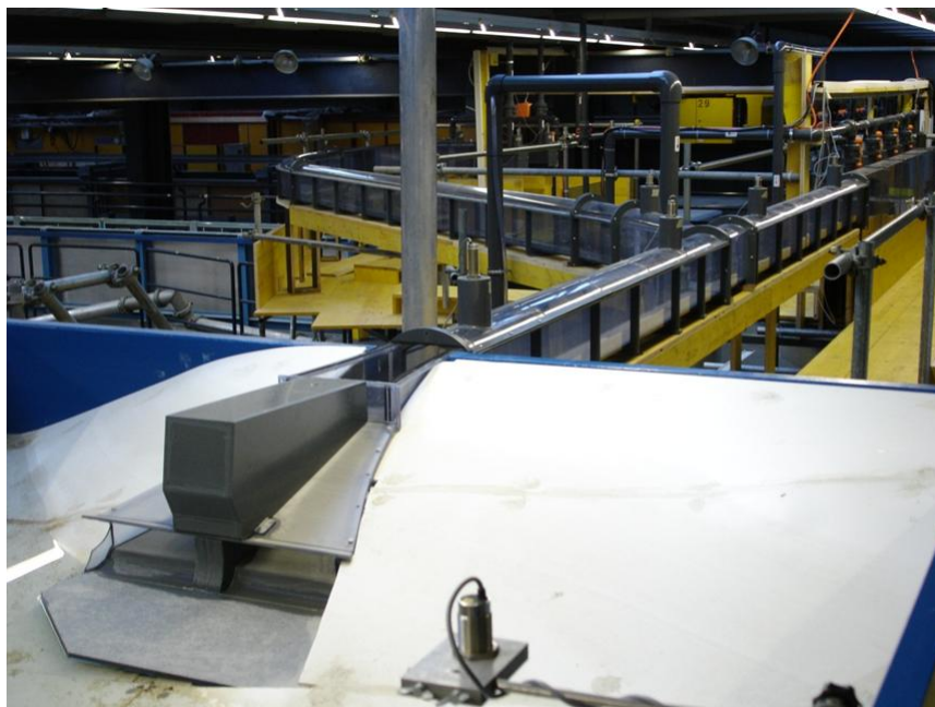
Figure 2 : Physical model of the FMHL+ tailrace channel at 1:30 scale
