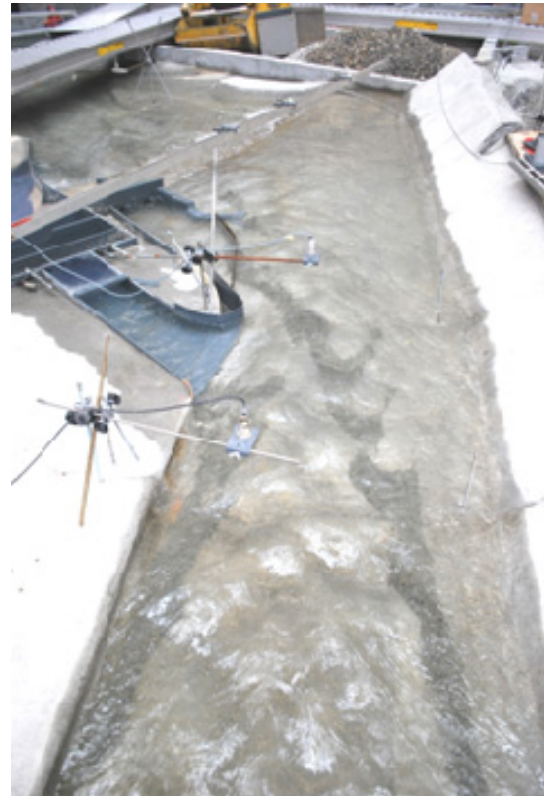
Figure 1 : Configuration 3 sans turbinage; comportement sédimentaire pendant la pointe de crue / Configuration 3 without turbining ; sedimentary comportment during peak flood
