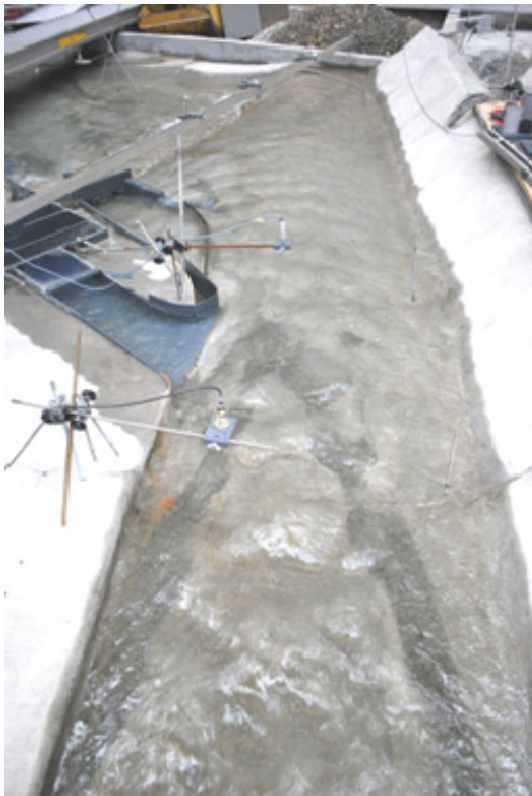
Figure 1 : Configuration 3 sans turbinage; comportement sédimentaire pendant la pointe de crue / Configuration 3 without turbining ; sedimentary comportment during peak flood
