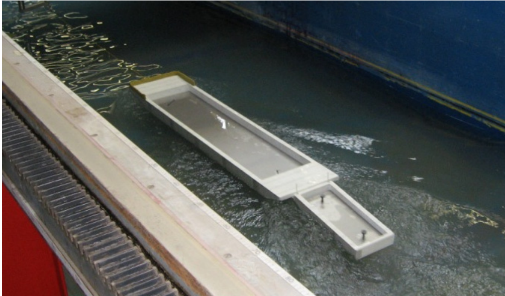
Figure 4 : Convoi tiré à 24 km/h ( V_{\text{prototype}} ) / Ships in convoy pulled at 24 km/h
