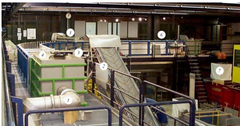
Figure 1: 1. Alimentation, 2. Tapis roulant (10 m), 3. Tapis roulant (2 m), 4. Répartiteur de sédiments, 5. Cadre de mesure, 6. Restitution, 7. Bac filtrant / 1. Inlet, 2. Conveyor belt (10 m), 3. Conveyor belt (2 m), 4. Sediment distribution, 5. Measurement frame, 6. Outlet, 7. Filtering basket
