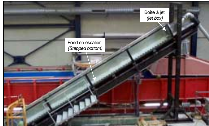
Fig. 2: Canal à forte pente (8m de long, 0.5m de large, pente de 30°) Steep flume (8m long, 0.5m large, slope of 30°)
