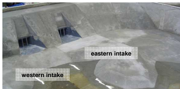
Figure 2: Hydraulic model of the two intakes
