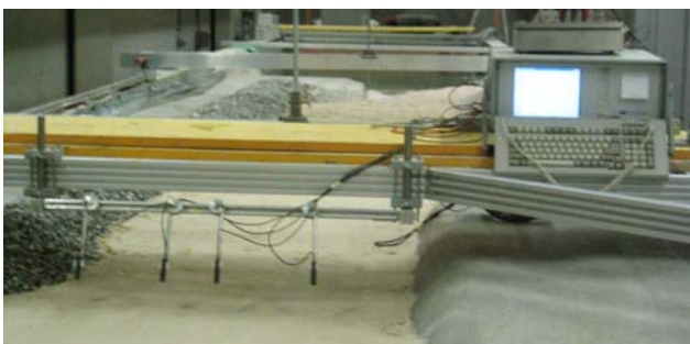
Figure 4 Physical model of the Rhone River with UVP transducers mounted on a measurement mobile frame.
