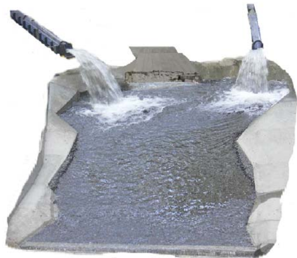
Figure 2 : Front view as a photomontage of the physical model and damaged dam toe
