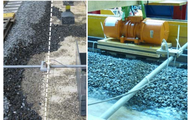
Figure 2: Left, test with 2 obstacles: catenary pole downstream of bridge pier; distance between obstacles 4.5 m, slope 3%. Right, test with vibrator, slope 0.65%, discharge 0.05 m 2 /s.
